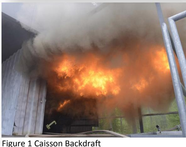
Figure 1 Caisson Backdraft
